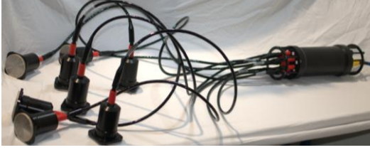
Figure 2 : Octopulse POD with 8 electrodes.
